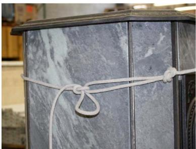
9. Remove the exterior stone panel. The furnace cement will make this removal difficult. If you rock the panel left and right as you lift it will help loosen the cement.
